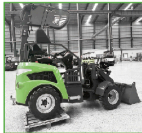
Joint center that can swing 12 degrees, better suited for rough
