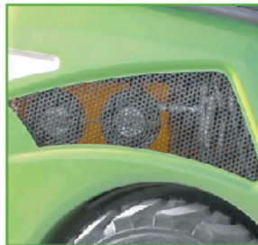
Hydraulic oil radiator, which can protect the machine
