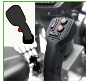
Electric joystick, ECO mode to help save energy
