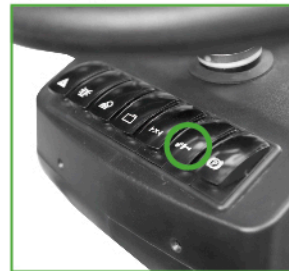
Quick hitch safety switch
