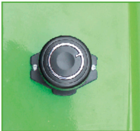
Hand throttle can help maintain a constant speed while working
