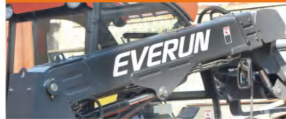
ONE-PIECE CASTING TELESCOPIC ARM
